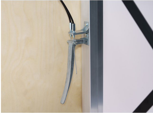
Bowden cable for releasing the pin (height adjustment)
